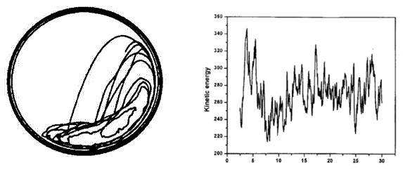
**Figure 6.**Trajectory of a single particle in cataracting **Figure 7**: Kinetic energy distribution Mode.
