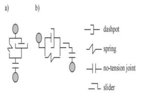
**Figure 1**.Contact model for DEM simulations in the (a) normal and (b) tangential directions.
