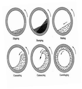
Figure 2: Schematic view of the different modes of solids motion (Boateng, [1993])
