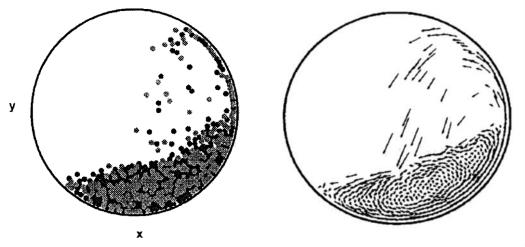
**Figure 4**. Granular solid bed during cataracting mode**Figure 5.** Velocity profile of the cataracting mode
